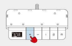
Use the "-" button to move the desk to the lowest position. Enter the Reset mode by pressing and holding the "-" button until the display shows "RST"; release the button (about 3 seconds).
