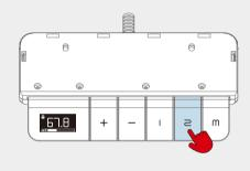
Use the "—" button to move the desk to the lowest position. Enter the Reset mode by pressing and holding the "—" button until the display shows "RST"; release the button (about 3 seconds).
